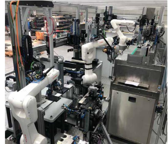
Together with our customer we analysed potentials for improvement compared to the predecessor systems. On the one hand, processes were optimised and on the other hand, proven functionalities were adopted. The assembly system is designed in such a way that manual intervention is limited to set-up, maintenance and material provision and removal. Since its commissioning, it has not only increased production capacity, but also offered the opportunity to utilise production more flexibly.
