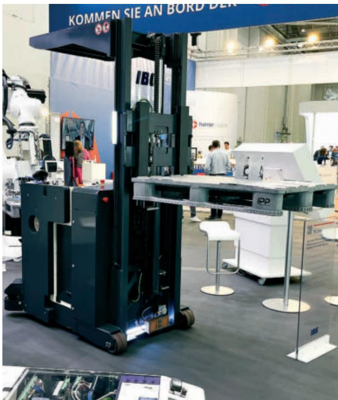
FC Lifter: autonomes, fahrerloses Gabelstapler-FTS | FC Lifter: autonomous, driverless forklift AGV
