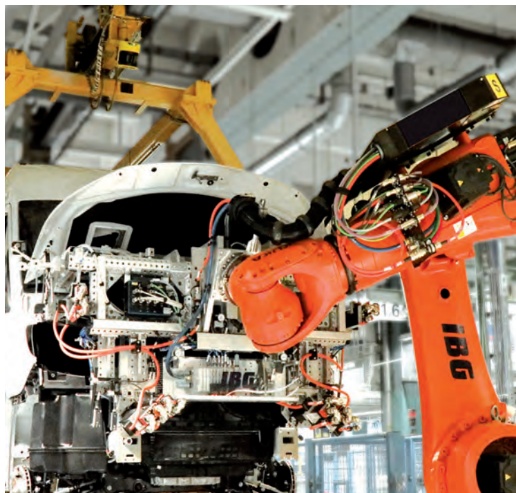
Frontendmontage: vollautomatische Verschraubung des Frontends. Frontend assembly: fully automatic bolting of the frontend.
