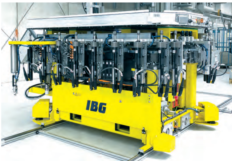
Hochvoltbatterie-Montage: simultane Verschraubung am Unterboden. High-voltage battery assembly: simultaneous bolting to the underbody.
